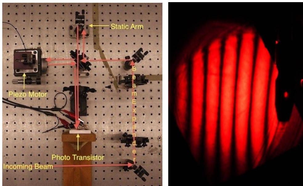
Figure 3. (Left) Interferometer-based motion encoder prototype, (Right) Sample Interference Pattern
