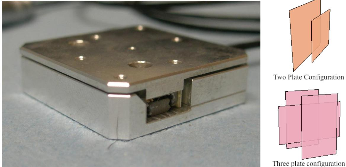
Figure 7. (Left) Image of the piezo electric motor stage, (Right) Two and three plate capacitor configuration
