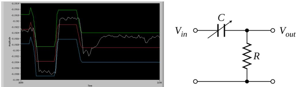
Figure 4. Current prototype of the capacitive sensor feedback loop for controlling motor position
