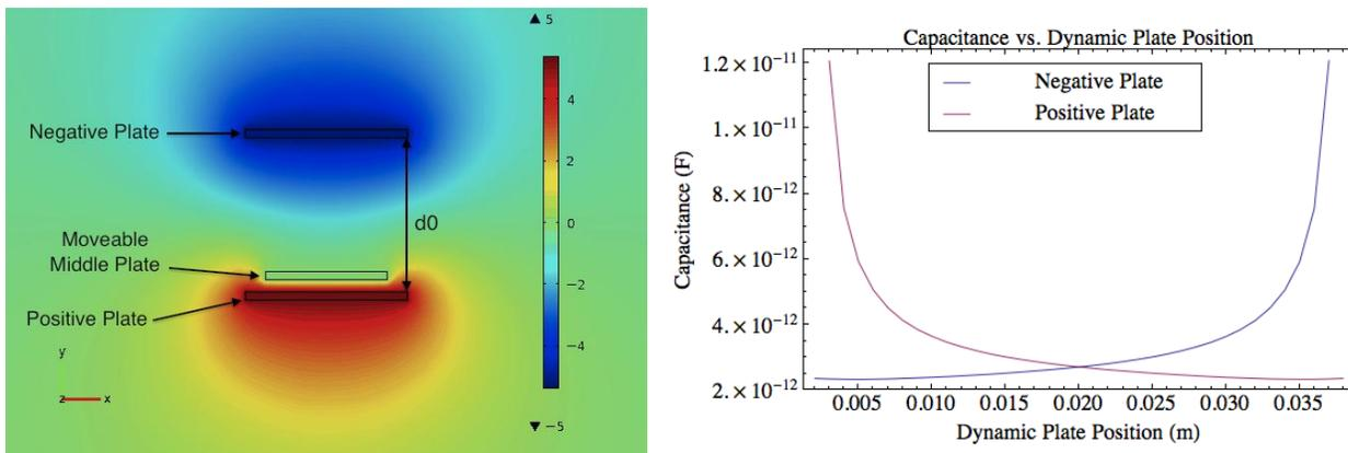
Figure 6. Simulated Three Plate Capacitive Distance Sensor Results
