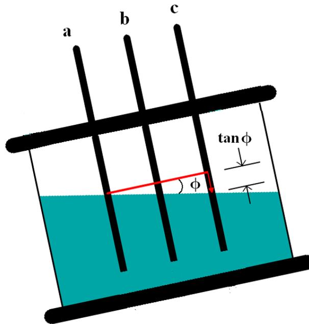
Figure 3: Cross-section of tilt sensor. The solution, always level to local vertical, is the shaded region while a, b, and c, represent aluminum electrodes.
