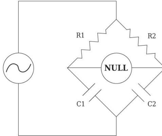
Figure 4: Capacitance bridge circuit.
