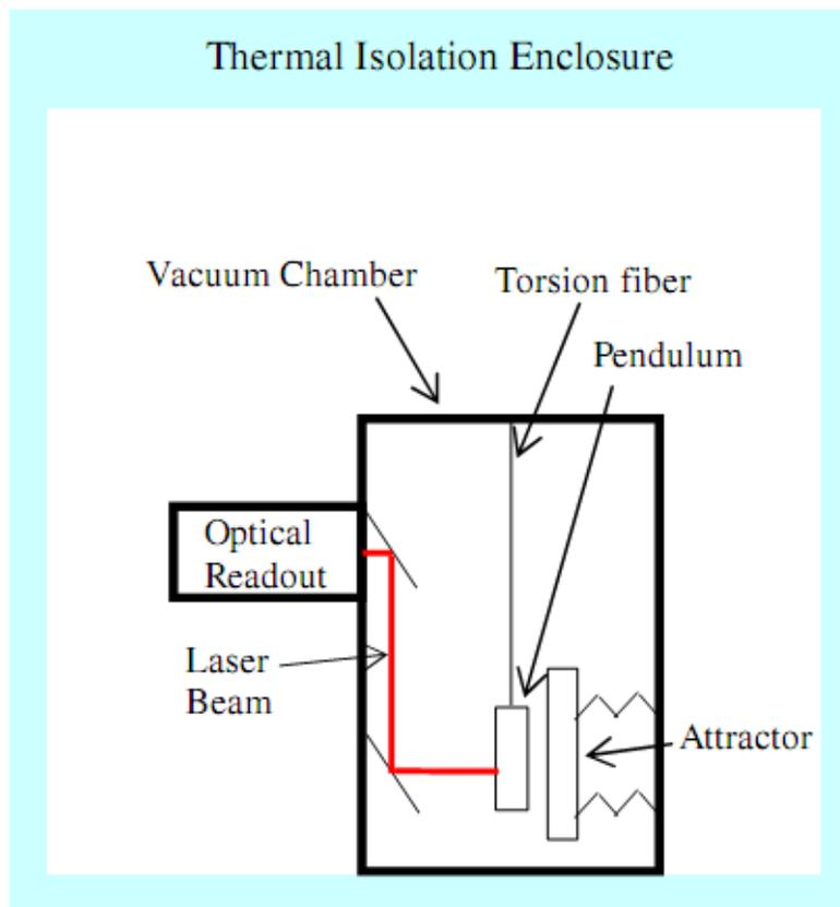
Figure 1: Cross-sectional view of apparatus.
